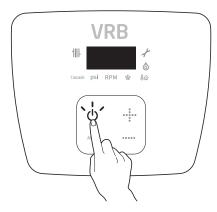
To view information about the boiler, press the MODE and ••••• buttons for 5 seconds.
