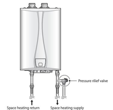
If the pressure relief valve discharges hot water periodically, thermal expansion may occur due to an expansion tank problem or small expansion tank size. Do not plug the pressure relief valve.
