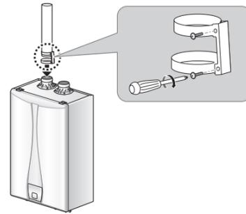
**Notice** Tighten the screws and fix the vent clip.
