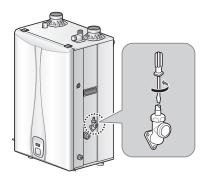
8 Close the drain valve when the water is completely drained.
