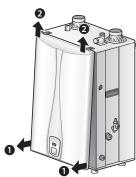
4 Remove the air intake filter located under the air intake connector.
