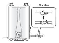
4 Turn off the water supply valve on the inlet to the water heater.
